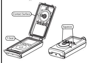
To ensure the T-Seal is fully seated in the base of the housing, firmly squeeze on both sides of the housing after each insertion of the player. Always check to make sure the latch is closed and locked prior to use.
